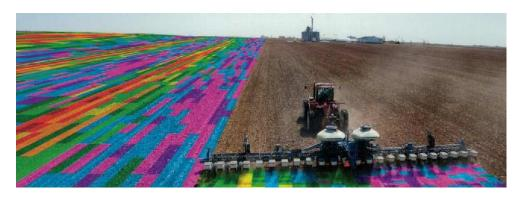
Your downforce on each row unit is also very important in these minimum-till scenarios. Controlling the downforce as well lifting the units can be done very quickly row by row. DeltaForce is the proven leader in hydraulic downforce control. Your planter will be able to function in any field condition and automatically sense the downforce
